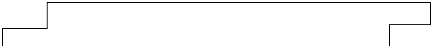
1 x 8 PRIMED REVERSABLE NICKEL GAP (Actual size \frac{3}{4} " X 7 \frac{1}{4} ") * WOSN8TR - 1- SIDE SMOOTH 1-SIDE ROUGH SAWN
