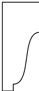
32 PWP * 1\frac{1}{16} " x 1\frac{5}{8} " Barge Mould
