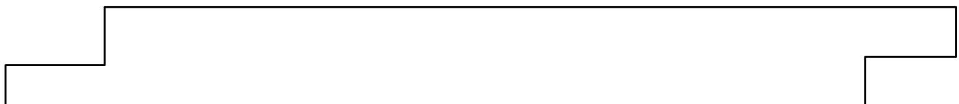
1 x 8 PRIMED REVERSABLE NICKEL GAP (Actual size \frac{3}{4} " X 7 \frac{1}{4} ") * WOSN8TR - 1- SIDE SMOOTH 1-SIDE ROUGH SAWN
