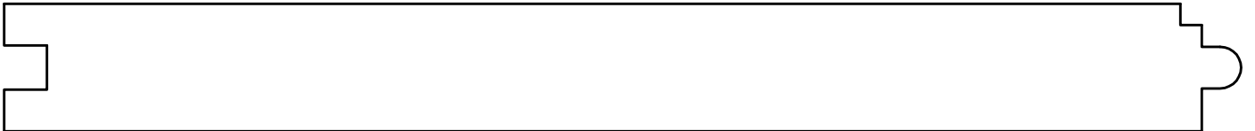
24224-QRK-TAG \frac{3}{4} " x 7" (face) Tongue & Groove
